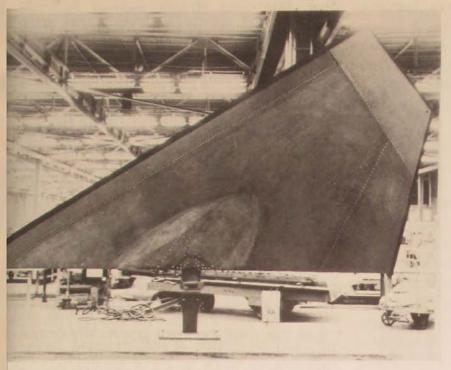
The F-4 rudder has engaged the cooperative efforts of AFML, McDonnell Douglas, and the AF Flight Dynamics Laboratory in comparing aluminum, beryllium, and boron composite structures. . . A horizontal stabilizer for the F-111 is the largest aerospace structure fabricated of boron composite to date, the boron structure saving 300 pounds over the current aluminum part.
