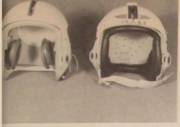
Compared to the standard issue helmet, the AFML custom helmet fits better, has only four inside pieces, and weighs less. . . . The photomicrograph (below) shows fiber orientation in a composite material reinforced with boron/epoxy tape.
